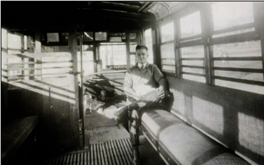
Walter Johnson, Jr. sits proudly in one of the three buses he and his brother Bob operated between Bloomfield and Newark. The slippery rattan seats, duck board floors and open-window "air-conditioning" were standard equipment on public transportation of the time. The bars on the windows were a safety feature designed to prevent curious sightseers from losing their heads through contact with a passing vehicle. Photo courtesy of Joseph Barry.
